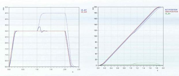
*Comparison of lag distance with and without MR controller. Without the MR controller, the lag distance increases from 3 mm to 4.5 mm (dotted line) due to the influence of an external force. MR control compensates for this.*
